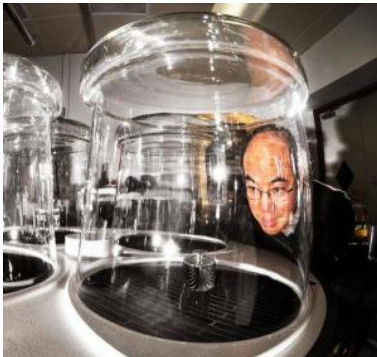
Hy Tran examines a kilogram sample in a mass comparator at Sandia's Primary Standards Laboratory. (Credit: Photo by Randy Montoya)
