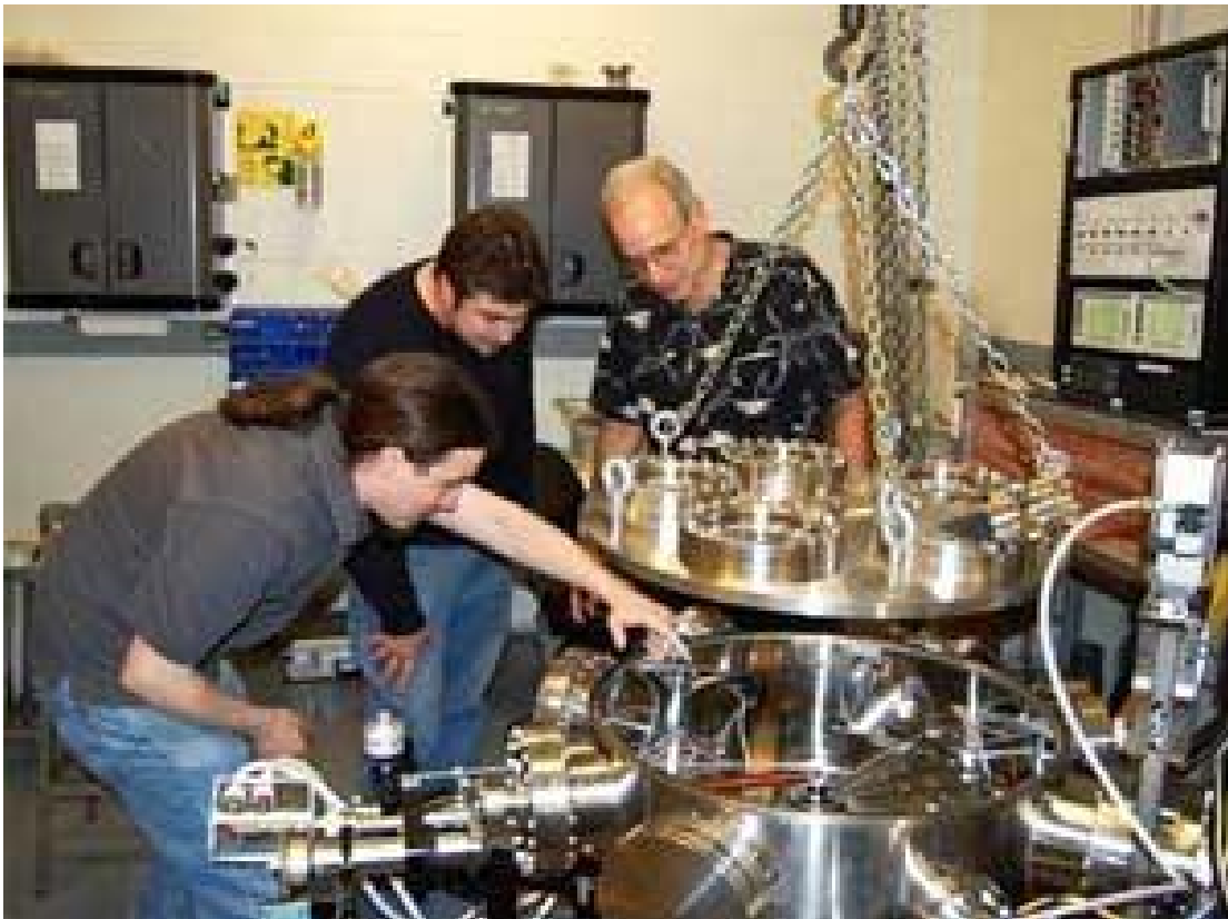
Graduate students Dan Casey and Mario Manuel, left, and Professor Richard Petrasso of the MIT Plasma Science and Fusion Center with the detector used to study implosions that recreate the high temperatures and densities found inside stars. (Credit: MIT photo by Sean McDuffee)
